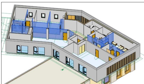
A cloison placostil 98 sèche
